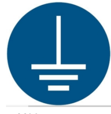
M005 – Grounding required
