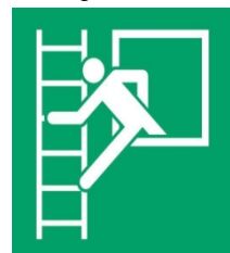
E016 – Window with emergency ladder
