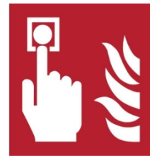
F005 – Fire alarm point
