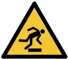
W007 - Tripping hazard
