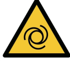
W018 - Automatic start hazard
