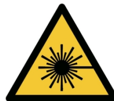
W004 - Laser radiation hazard
