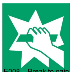
E008 – Break to gain access
