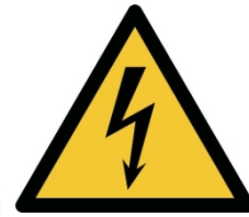
W012 - Danger: electricity
