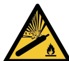
W029 - Pressurized cylinder hazard
