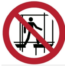
P025 – Do not use scaffolding inc.
