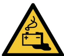
W026 - Danger: battery charging
