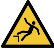
W008 - Danger of falling with uneven ground
